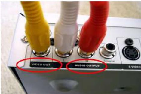
**Note:** Be sure to plug an RCA-3 color-coded cable into the Video or A/V Out section on the rear of the VCR.
